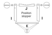
Hold the 'position stopper' facing the front of the chair and set it upright into the first reclining position above the back of the chair. Slat (K) should sit perfectly in the notch. Turn the upper back support (J) so that the notches are facing the front of the chair.
