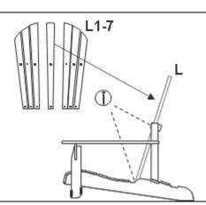
Secure all slats in the right order underneath the low back support (D). Use one 4x40 mm screw per slat. Do not tighten the topmost screws yet. First, spread out all the slats so that they form a nice curve at the top and so that they are evenly spaced. Use the notches as reference points. When all slats are correctly positioned, the last 4x40 mm screws can be tightened up.
